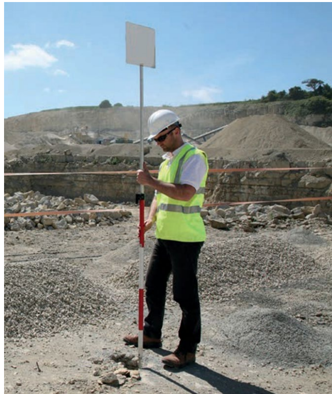
Figure 40 Target on survey pole being used to position a hole collar
